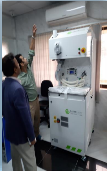
Fuel Cell Test Station(Green light)
